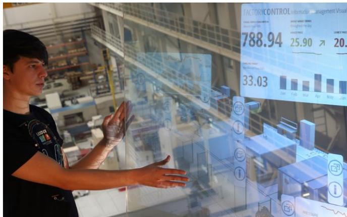
**Image:** All data of resources needed, such as compressed air, water, electrical energy, and machines and process data come together at the factory level in the „Control Center“. Scientists can visualize the information in real time on a dashboard and can thus design processes to save energy and raw materials. The transparent glass monitors are reminiscent of “holodecks” and can be controlled by means of gestures.
