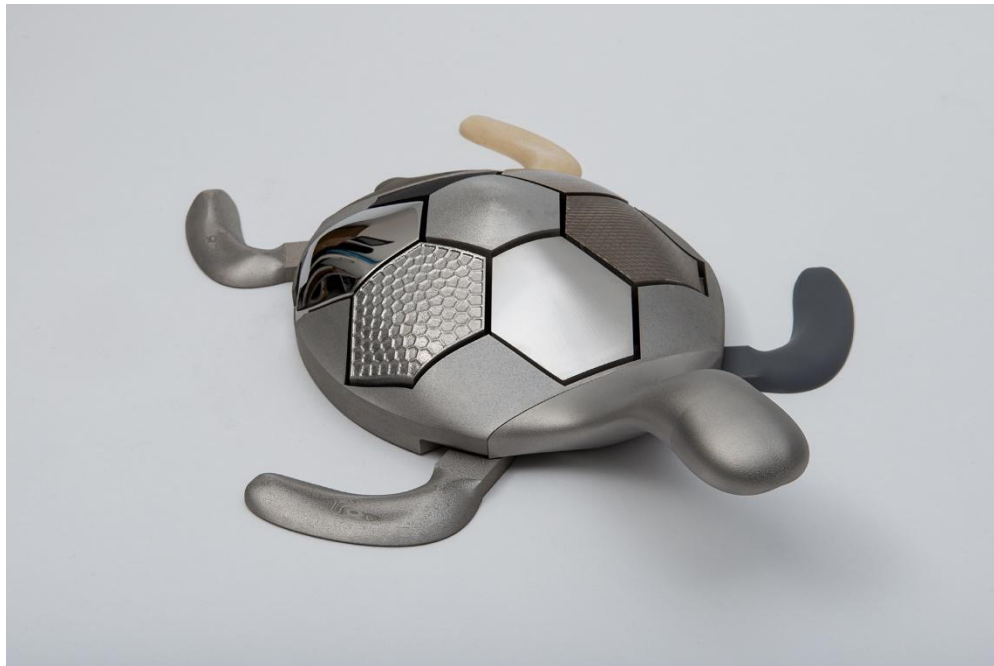
Fig. 1: Additive manufacturing processes typically produce semi-finished products that only become high-quality end products through post-processing. The turtle at the Fraunhofer exhibition booth makes this principle visible and tangible. © Fraunhofer IPT
